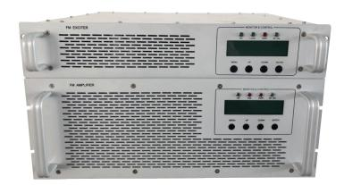
**POS-2000** is FM transmitter for broadcasting, able to transmitter in the band between 87.5 to 108 MHz, Continuously adjustable output power from 0 up to 2500 watt. Completely microprocessor-controlled easy to program from the menu, all main parameters can be read on the large LCD display. They are designed with aluminum box to be contained in a 19" rack of 6U.
